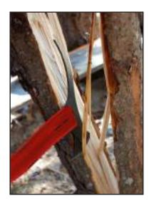
**Using the cutting edge:** to cut remaining wood fibres on split logs. Suitable to **knock off smaller branches**. To lift light, cut in length chumps as well as to clean up smaller and light pieces of wood, as well as for **universal use in recovery vehicles**.
